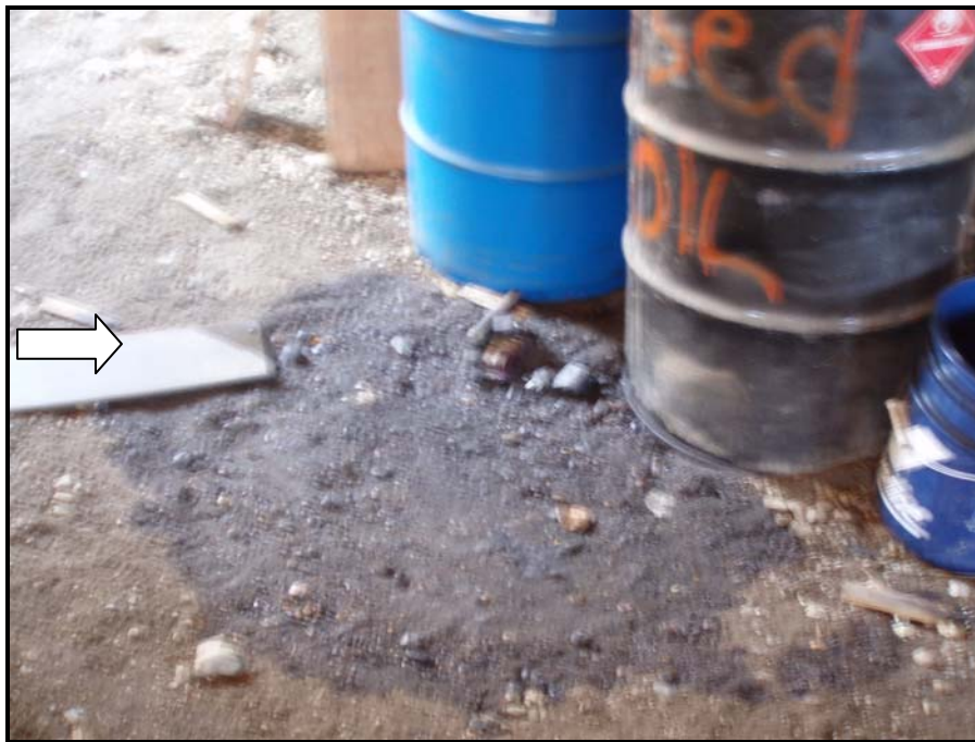
Photograph 18: Area of stained soil associated with used oil barrels inside Section 2 of the City Shop.
